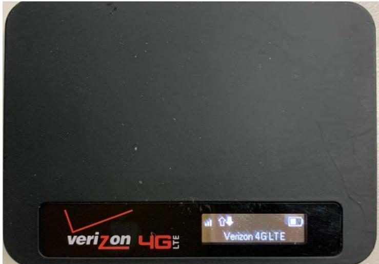
To see the name and password of your hotspot connection, gently push the power button to cycle to the screen that has that information. You may need to press several times.
